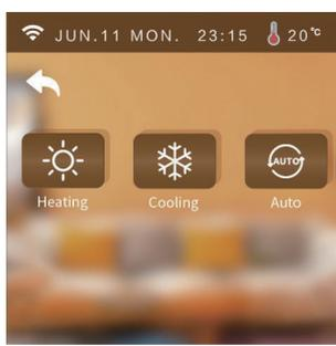
**Note:** Enter the password "168" in "Parameter" and set the heating & cooling type by modifying N02.
